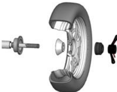
Main shaft → suitable cone → wheel → bowl → quick nut
